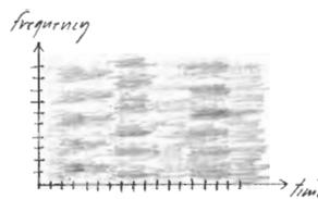
**Figure 4.14:** Spectrogram of a speech segment. 64 frequency bins are evaluated between 0 and 4 KHz, and a triangle window with 50% overlap is used.
